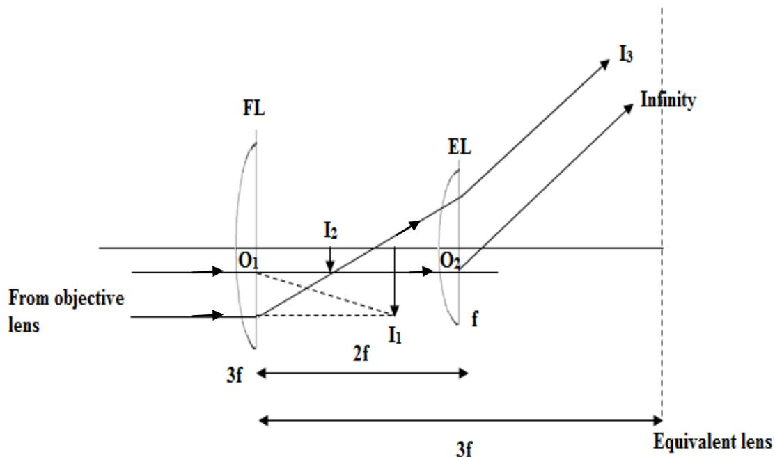
FL is the field lens of focal length  $f_1 = 3f$  and EL is the eye-lens of focal length  $f_2 = f$ . the distance between them is  $d = 2f$ . Light rays coming from the objective from the objective lens will form an image  $I_1$  in the absence of the field lens.  $I_2$  is the image formed by the field lens. This image is at the principal focus of the eye-lens. Therefore the emergent rays are parallel and the final image is formed at infinity.
