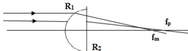
The more curved surface R1 is in the object side and the less curved surface R2 is in the image side. To some extent, it is a better method of minimizing the deviation. But the spherical aberration cannot be completely eliminated.
